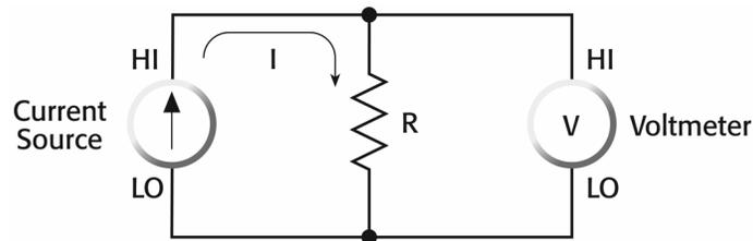
Figure 1—FVMC configuration for low-impedance devices
