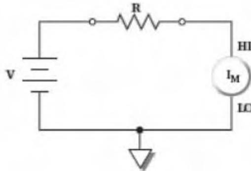
Figure 3—FVMC configuration for high-impedance measurement
