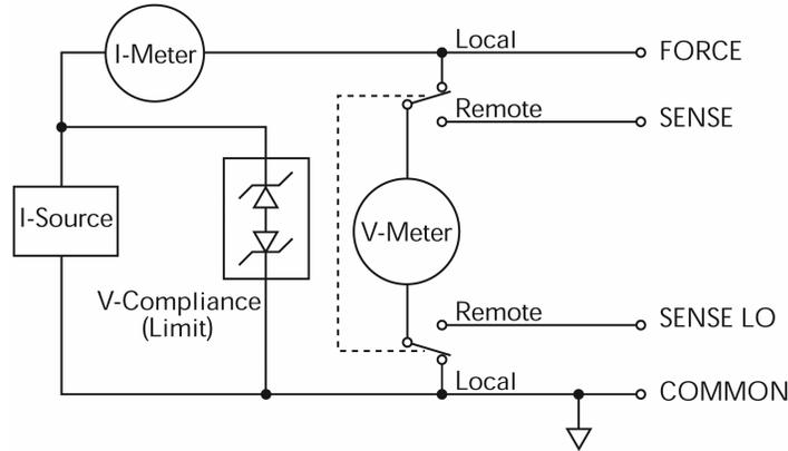
Figure 2—Remote and local sensing configurations
